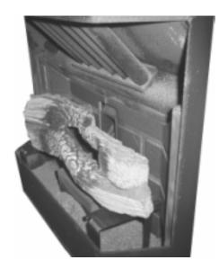
2 Remove the firepot from the pellet stove. Center the log shelf assembly (with extender attached) over the burnpot holder. Replace the burnpot. Place the log on the log shelf extender. When in place, the log should appear as shown in the photograph to the right.
